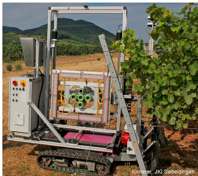
Fig.1: PHENObot consisting of a robotic platform, a multi-camera-system and a geo-information system.
